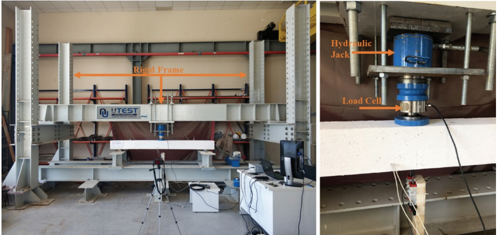
Figure 3 - Overview of test setup (left) and instrumentation for experiments (right)
