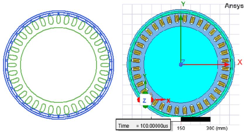
Fig. 1. ANSYS models of the designed generator
