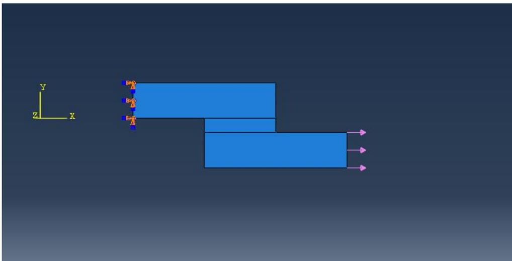
Fig. 7. Model showing boundary condition of the analysis
