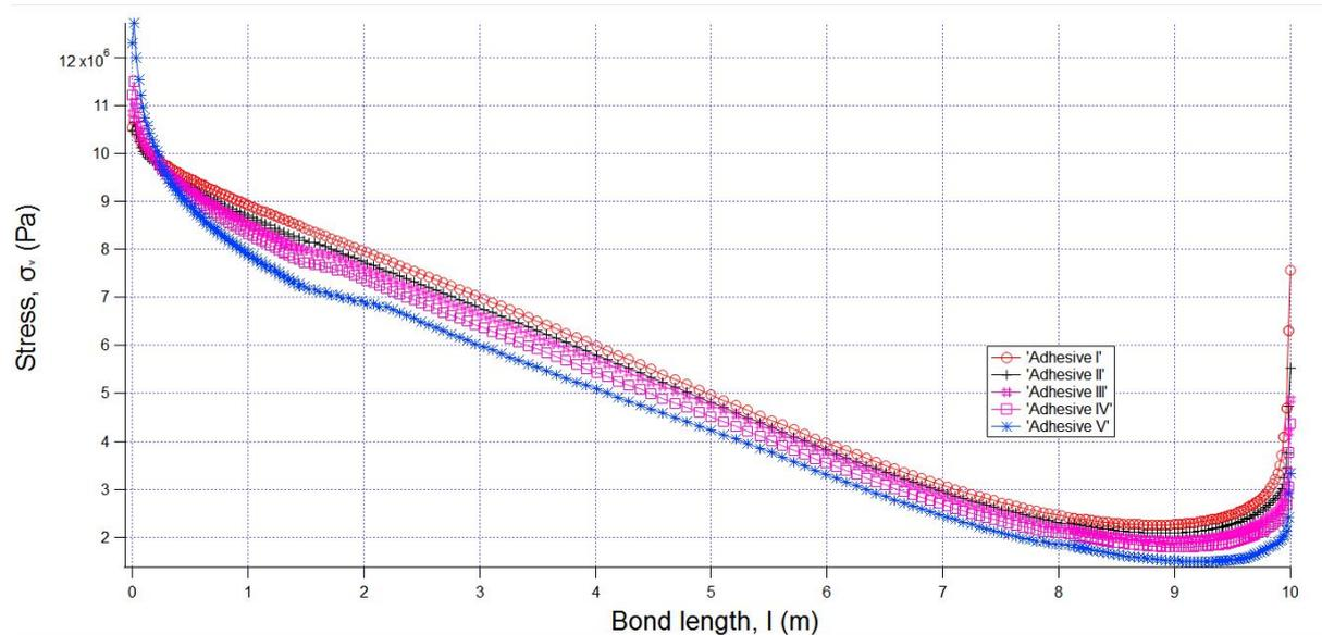
Fig. 10. Variation of Von Mises stress along the bond line of the adhesive bonded joint
