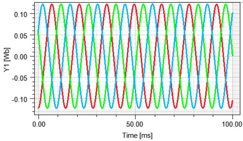
Fig. 7. Time-dependent graph of phase fluxes
