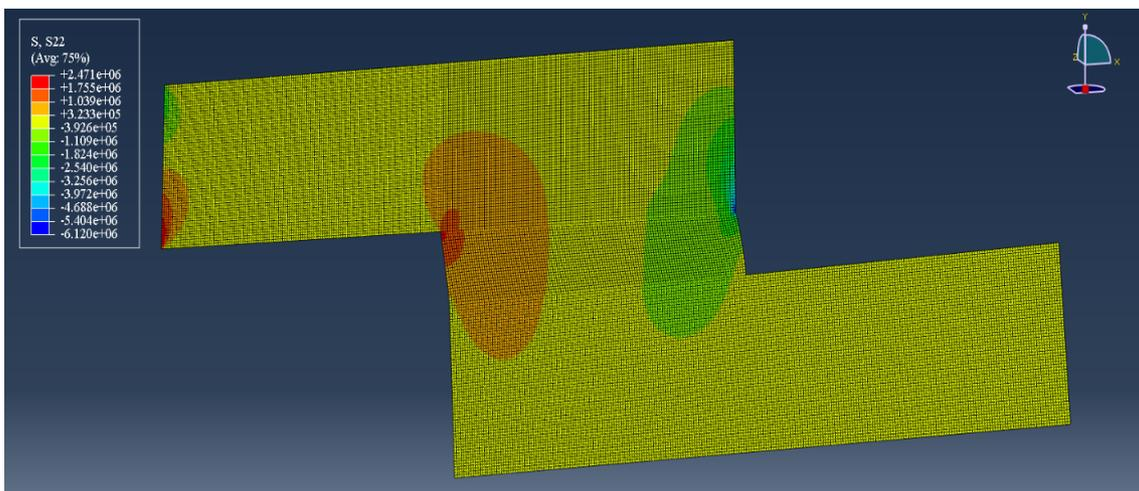
Fig. 15. Contour of displacement elements  $\sigma_{22}$  for adhesive I
