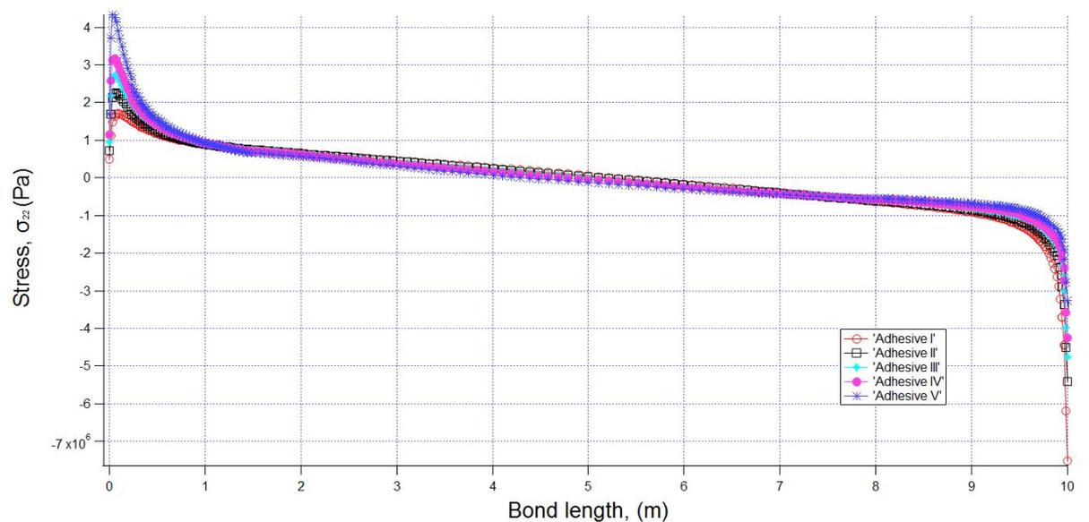
Fig. 9. Variation of  $\sigma_{22}$  along the bond line of the adhesive bonded joint
