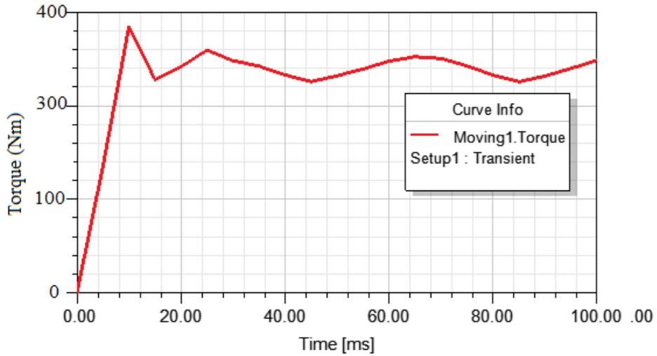
Fig. 4. Torque-time curve
