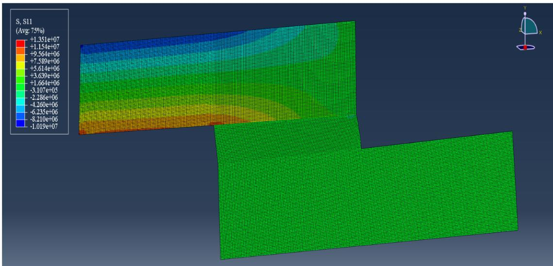
Fig. 14. Contour of stress component  $\sigma_{11}$  for adhesive I
