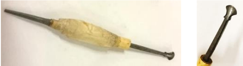
Photo 1-2: Yekşah Iron Tool (from bookbinding workplace of Islam Seçen)
