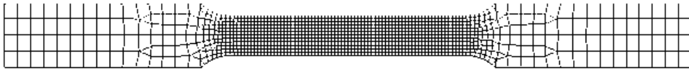
Figure 5. The finite element mesh of the ASTM E8 uniaxial tensile test specimen
