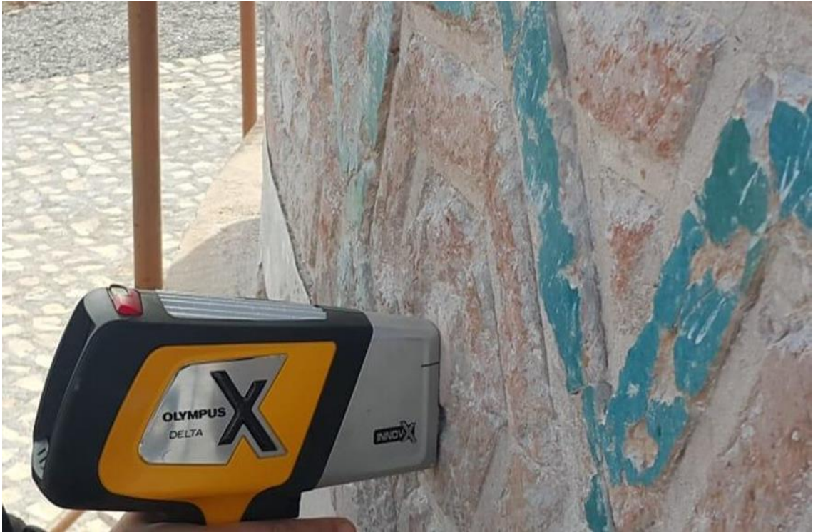
Figure 4. Analysis of the Unglazed Tiles of Zeynel Bey Tomb with P-EDXRF.
