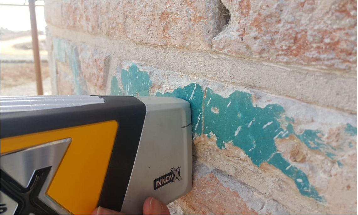
Figure 2. Analysis of the Light Blue Tiles of Zeynel Bey Tomb with P-EDXRF
