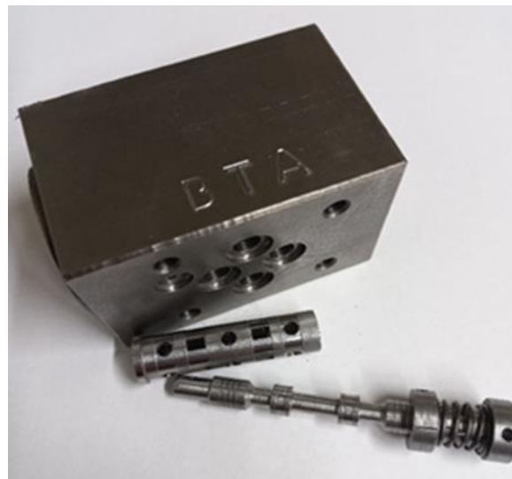
Fig. 2. Photograph of the disassembled valve.
