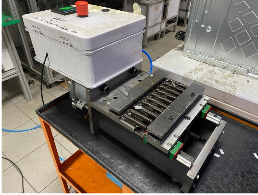
Figure 7. The extension spring fatigue machine after manufacturing and mounting (İmalat ve montajdan sonra uzatma yayı yorulma makinesi)
