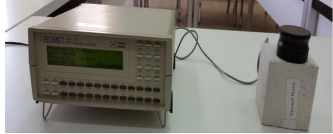
**Figure 1.** The thermal properties analyzer device
