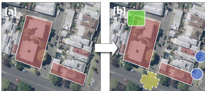
Figure 2. Not all property interests fit comfortably in the parcel framework: object-oriented design is required [3]; (a) actual cadastre, (b) cadastre of the future or Cadastre 2034.
