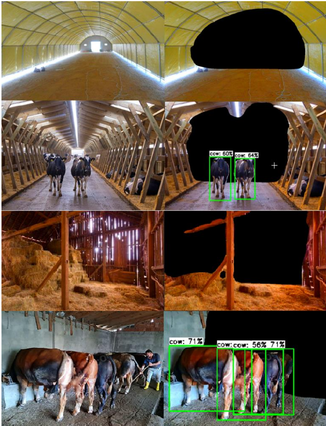
Figure 3. Images with depth estimation, in which only close objects are obtained, with object detection on it. On the left are the original images, on the right are the images with depth perception and object detection applied in the application.
