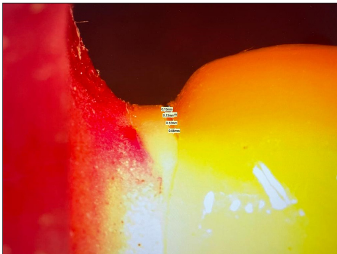
Figure 4. Marginal gap measurement under stereomicroscope.
