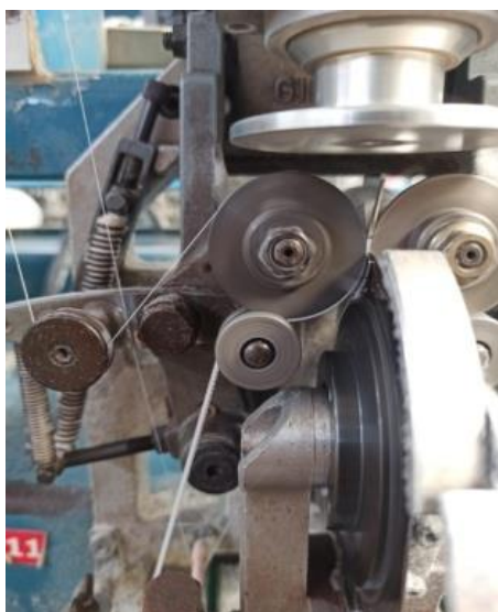
Figure 4. Adding fusible yarn to chenille yarn production
