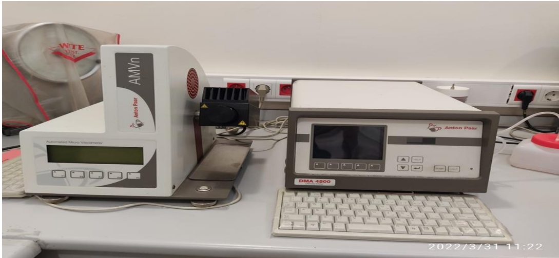
Şekil 1. Anton Paar Automated Micro Viscometer AMVn ve Anton Paar DMA 4500 Density Meter
