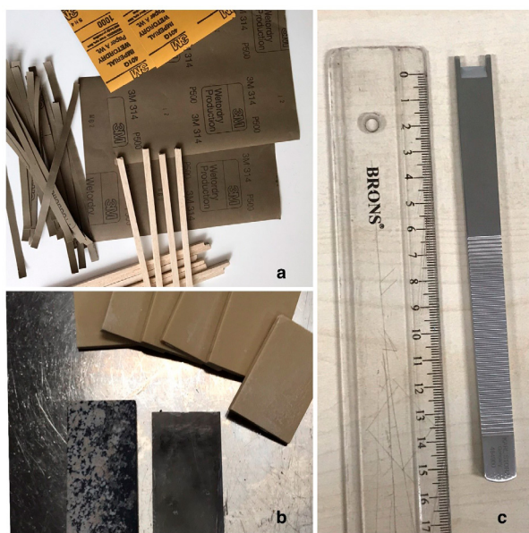
Figure 1: a) Sandpaper with 500 and 1,000 grit, cut into 10 mm thin strips and waiting to be bonded to wooden blocks for sharpening; b) Fine and c) Arkansas stones (shown as >>) with 500 and 1,000 grit and artificial bone blocks (*); and c) 10 mm Cinelli osteotome (Karl Storz, Tuttlingen, Germany).
