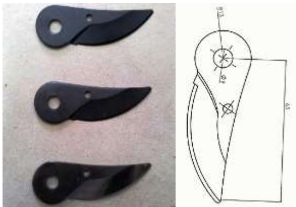
Figure 2. The pictures of the materials used in the construction of blades.
