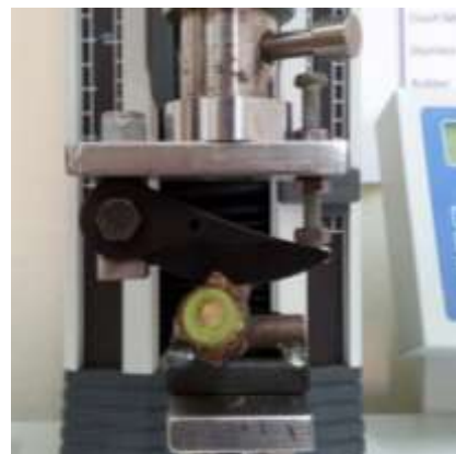
Figure 3. The testing system for the lopper blades (left view).
