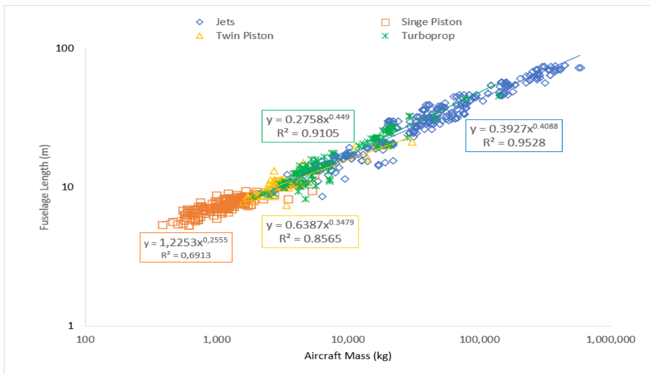
Figure 1. Representation of power correlation between fuselage length and aircraft mass on a base 10 logarithmic scale for different engine types.
