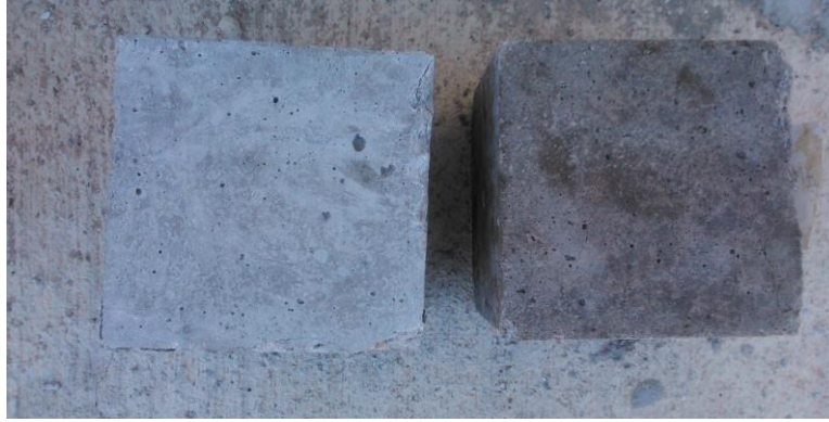
Figure 2. A concrete sample produced with limestone aggregate on the left, concrete sample using limestone, basalt and recycled asphalt aggregates together on the right.
