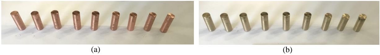
Figure 1. Turned electrodes prepared for EDM: (a) Copper (b) brass
