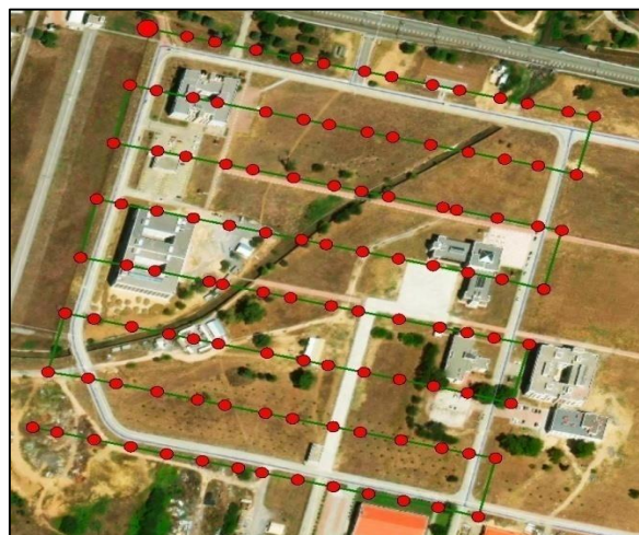
Figure 7. Imaging Plan for flying height of 120 meters
