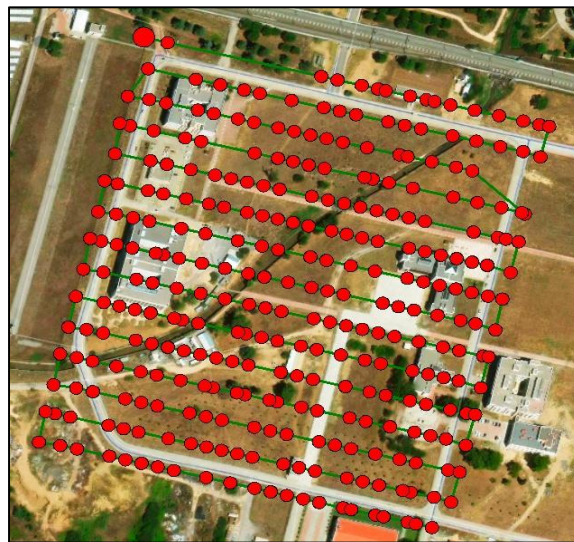
Figure 6. Imaging Plan for flying height of 60 meters altitude
