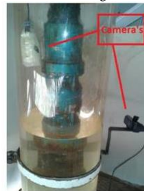
Figures 9 Submersible pump and connection of the camera
