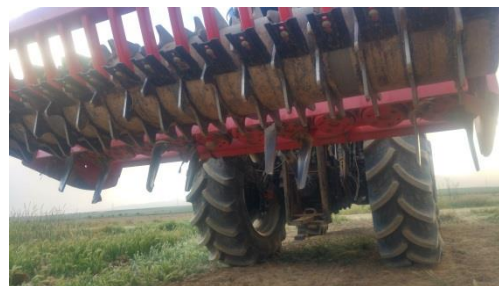
Figure 2 Modified vertical shaft-tiller (MVST)
