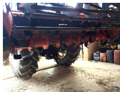
Figure 3 Modified horizontal shaft-tiller (MVST)
