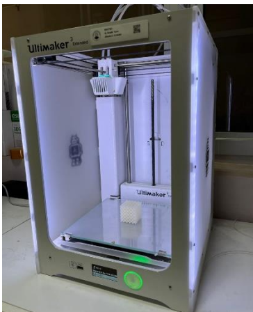
Figure 2. Manufacturing of lattice specimen with the 3D printer.
