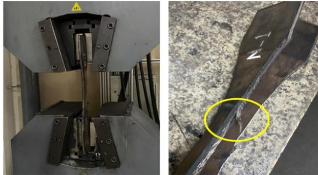
Figure 10. Breaking of specimen N-1 after tensile test.
