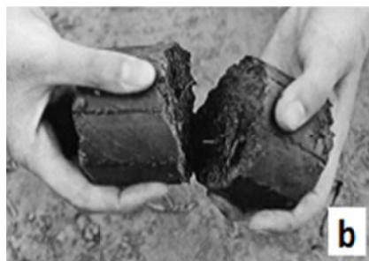
Fig.8. (a) Root auger for obtaining soil cores; (b) breaking a 10-cm long soil core to count the roots at the breakage faces (Reynolds et al., 2001).
