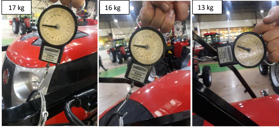
Figure 8. Springless ROPS mechanism force measurements
