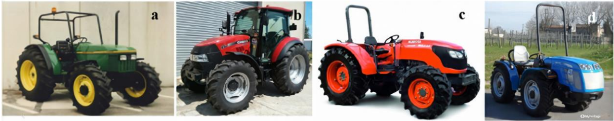
Figure 1. Tractor ROPS; (a) four-post frame, (b) cabin, (c) rear two-posts, (d) front-folding two-posts (Rondelli et al., 2018)
