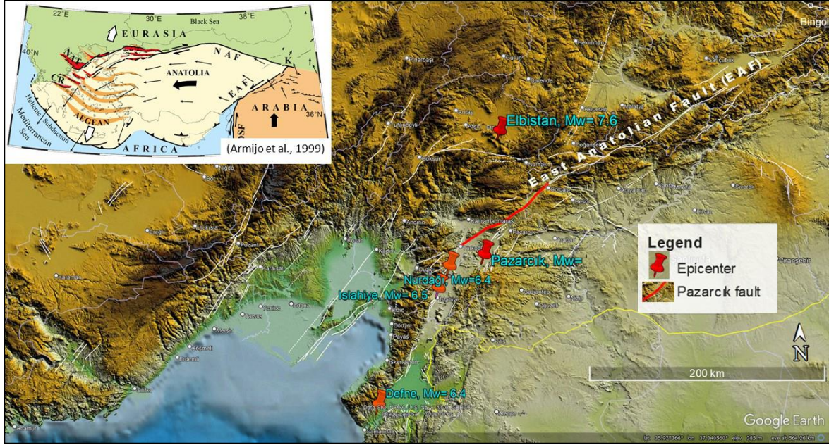
Figure 1: Anatolian plate and main tectonic lines (in small frame) (Armijo et al., 1999), East Anatolian Fault (EAF) (MTA, 2023 ve ATAG, 2023), Pazarcık segment (red line) (Karabacak et al., 2023), locations of February 06, 2023, and February 20, 2023 earthquakes (AFAD, 2023; Kürçer et al., 2023b; Utkucu et al., 2023).
