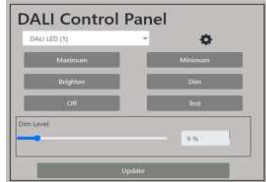
Fig.23. DALI Control Unit User Interface
