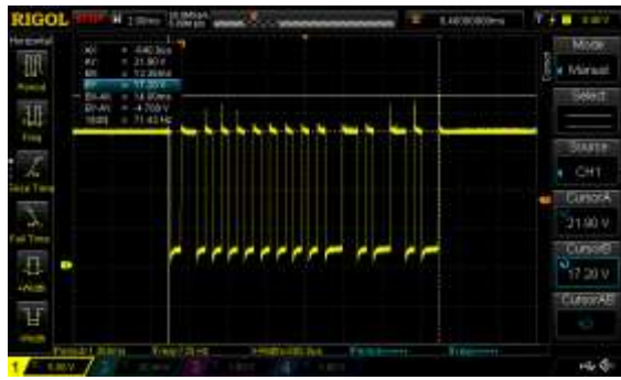
Fig.17. Observing Peaks at a High Level of the DALI Signal.
