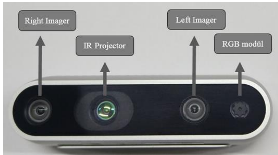
Figure 1. Intel® RealSense™ D435 Camera
