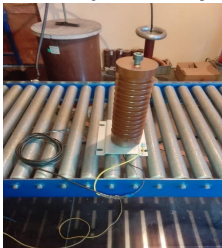
Figure 9. The final state of the designed transformer
