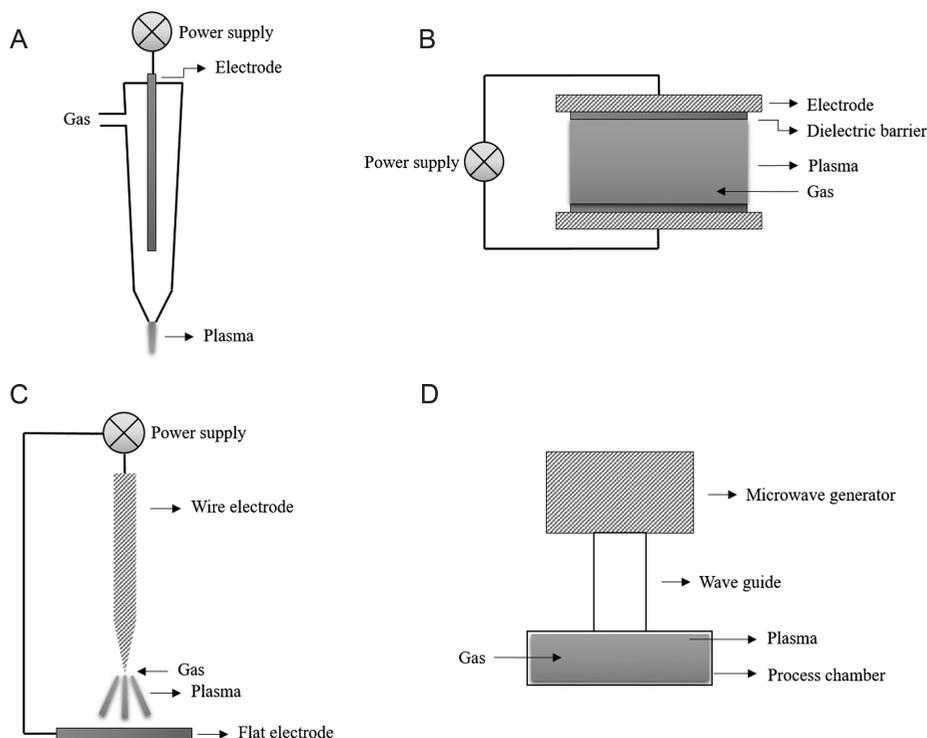
**Figure 1.** Different Cold Plasma Systems: (A) Plasma Jet, (B) Dielectric Barrier Discharge, (C) Corona Discharge, and (D) Microwave Discharge (Modified from Coutinho et al., 2018; Misra et al., 2016a; Surowsky et al., 2015).
