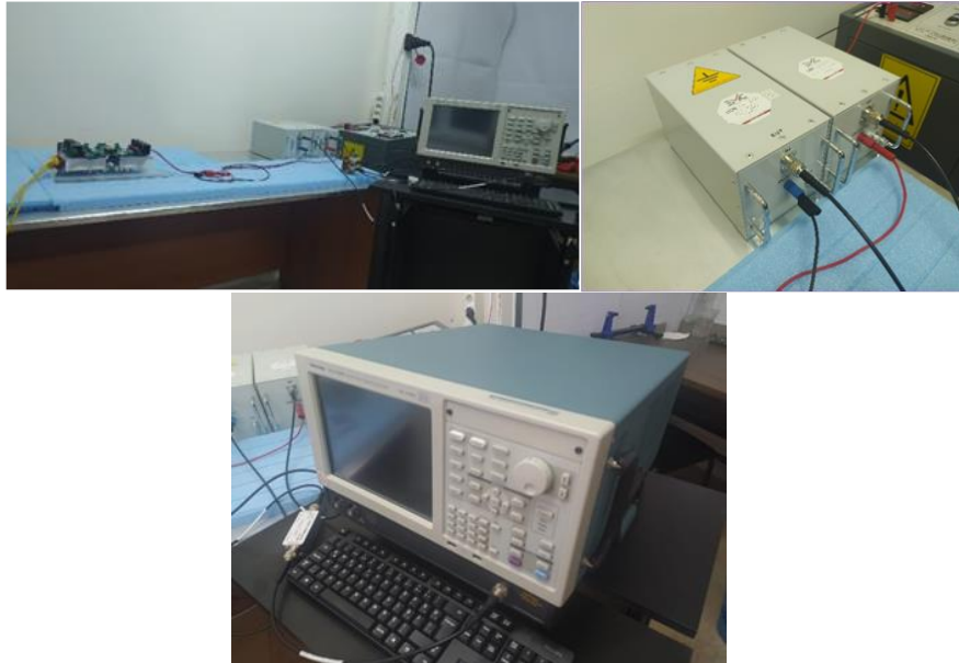
Figure 9: Conducted Emission Lab Test Bench, LISN and Spectrum Analyzer
