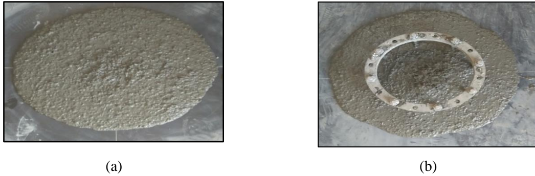
Figure 1. Fresh SCC tests: (a) Slump-flow, (b) J-Ring
