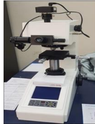
Figure 7. Vickers microhardness measuring machine [21].
