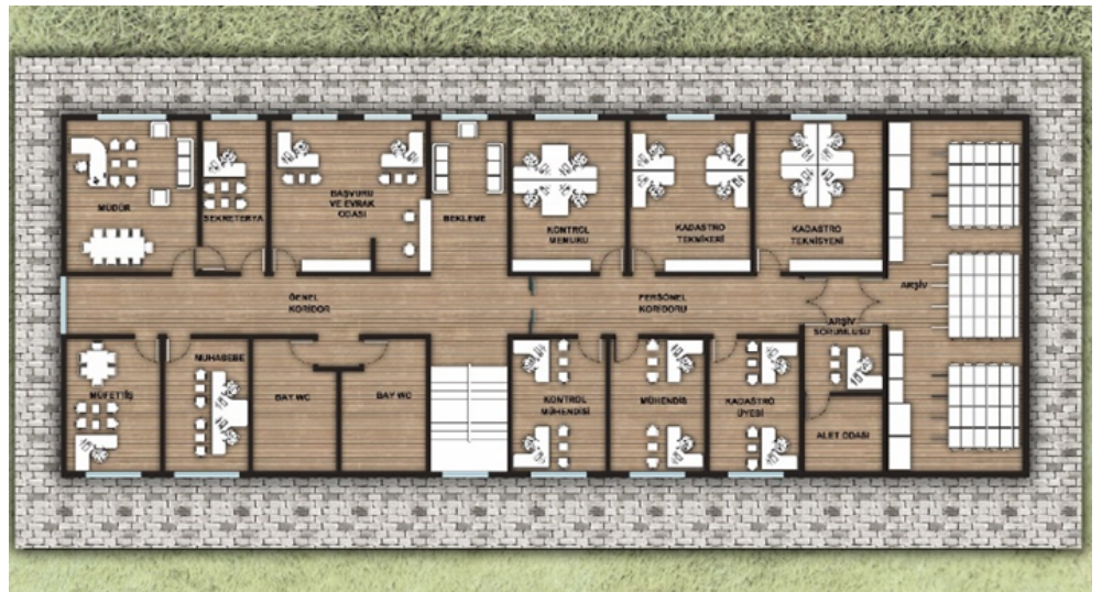
Figure 14. Example spatial design of Directorate of Cadastre (Archive of the General Directorate of Land Registry and Cadastre)
