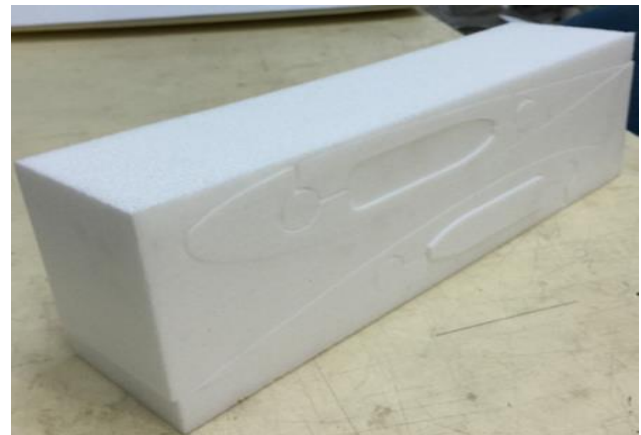
Figure 4. Obtaining the wing of the UAV from the CNC machine
