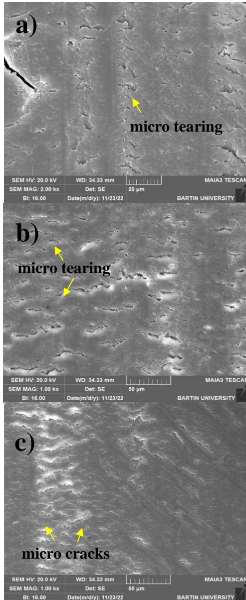
Figure 7. SEM images of the worn surfaces due to the load in composites produced with a “45” degree laying angle at a shear rate of 0.02 m/sec: a) 1 N, b) 3 N, c) 5 N.
