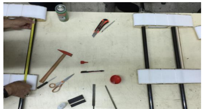
Figure 5. Threading the profiles of UAV into carbon pipes
