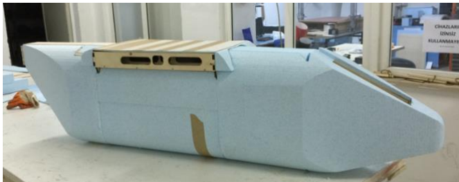
Figure 12. Covering the fuselage with foam
