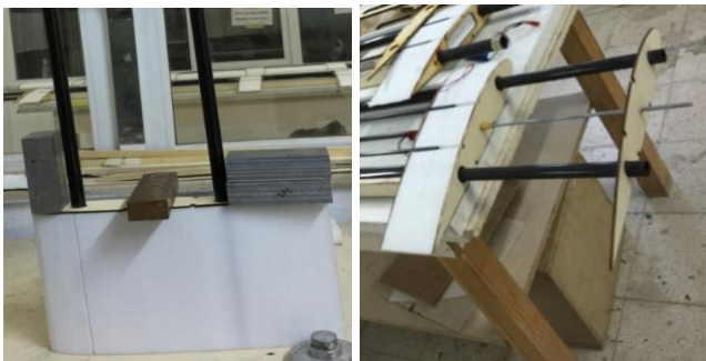
Figure 7. Installation of the morphing mechanism on the UAV
