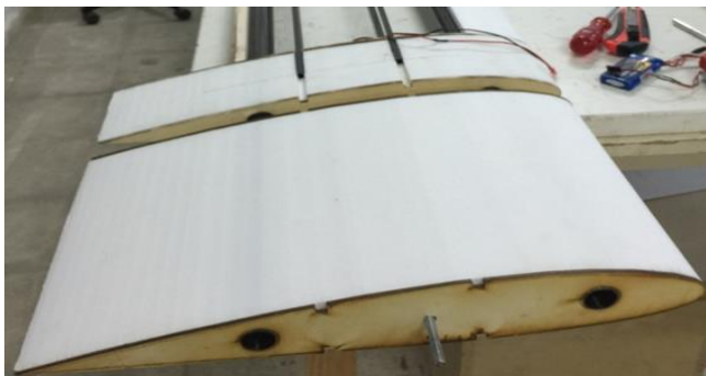
Figure 8. Installation of morphing mechanism on UAV
