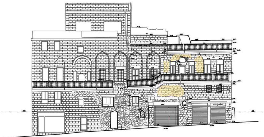
Figure 15. Material deterioration measured drawing of south façade
