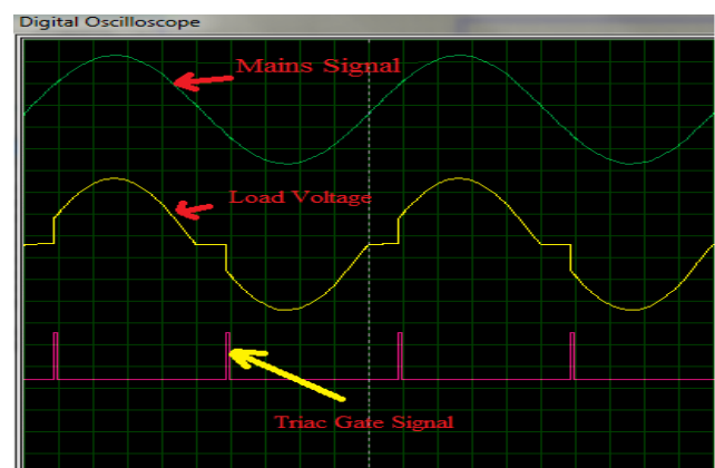
Figure 11. Oscilloscope measurements when triac is triggered at the beginning of the alternance.
