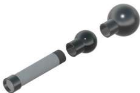
Figure 3. Whole Applicator 3D View with Two Different Spherical Tips
