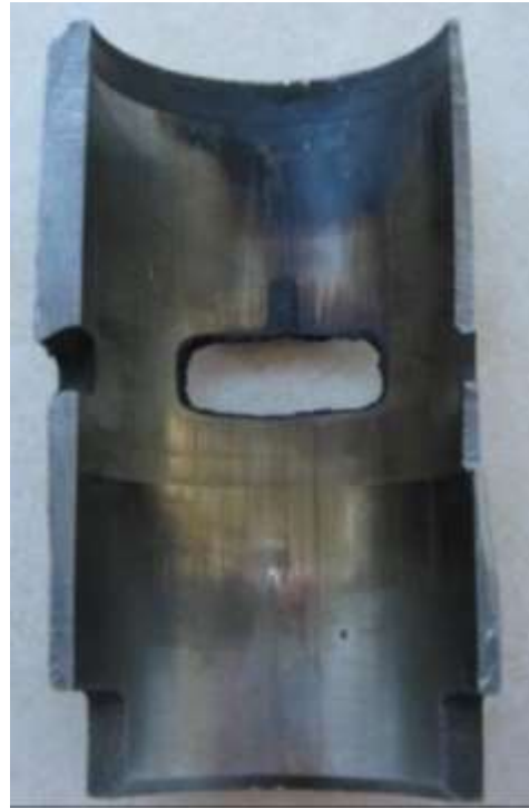
Figure 3. The surface of cylinder hazelnut oil was used as lubricant.
