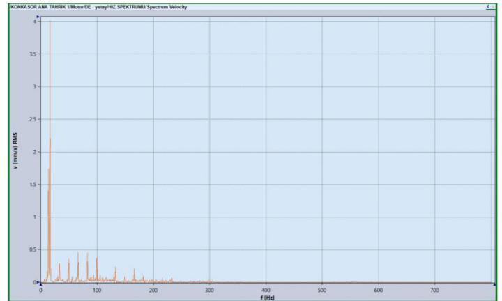
Figure 4. Crusher-1 Motor DE Horizontal Vibration Analysis
