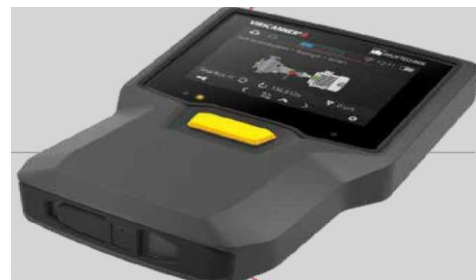
Figure 1. Vibration FFT Analyzer [16]
