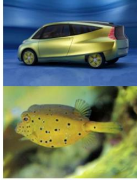
Figure 3: The first bionic concept vehicle by Mercedes- Benz inspired by boxfish (Yang et al., 2019)
