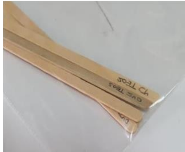
Figure 5. Final dried samples obtained by treatment with TEOS.
