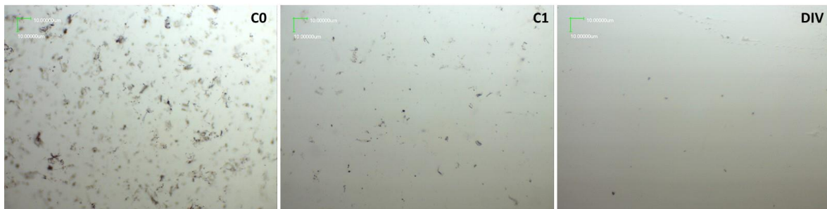
Figure 3. Micrographs of wastewater C0:Control, C1: Centrifuged Control, DIV:360 Watt and 60 Second MW irradiated
