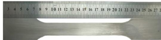
Figure 2. The tensile test specimen
