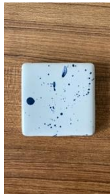
Figure 5. Faults due to splash of colored glaze.
