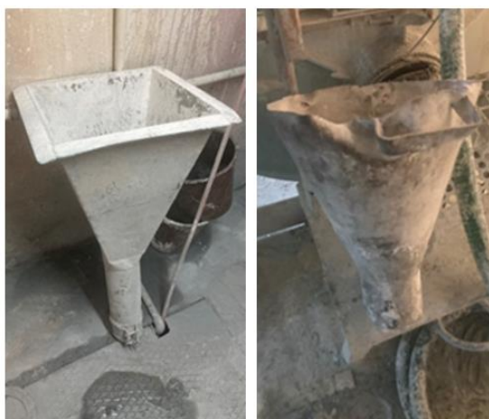
Figure 6. Hopper for raw material addition.
