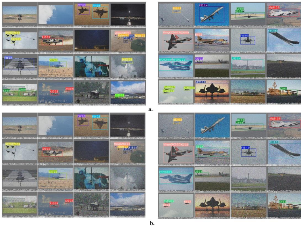
Figure 8. Examples of the YOLO detection on the 30%-Gaussian-Dataset and 50% Gaussian-Dataset. a. 30% noise, b. 50% noise.
