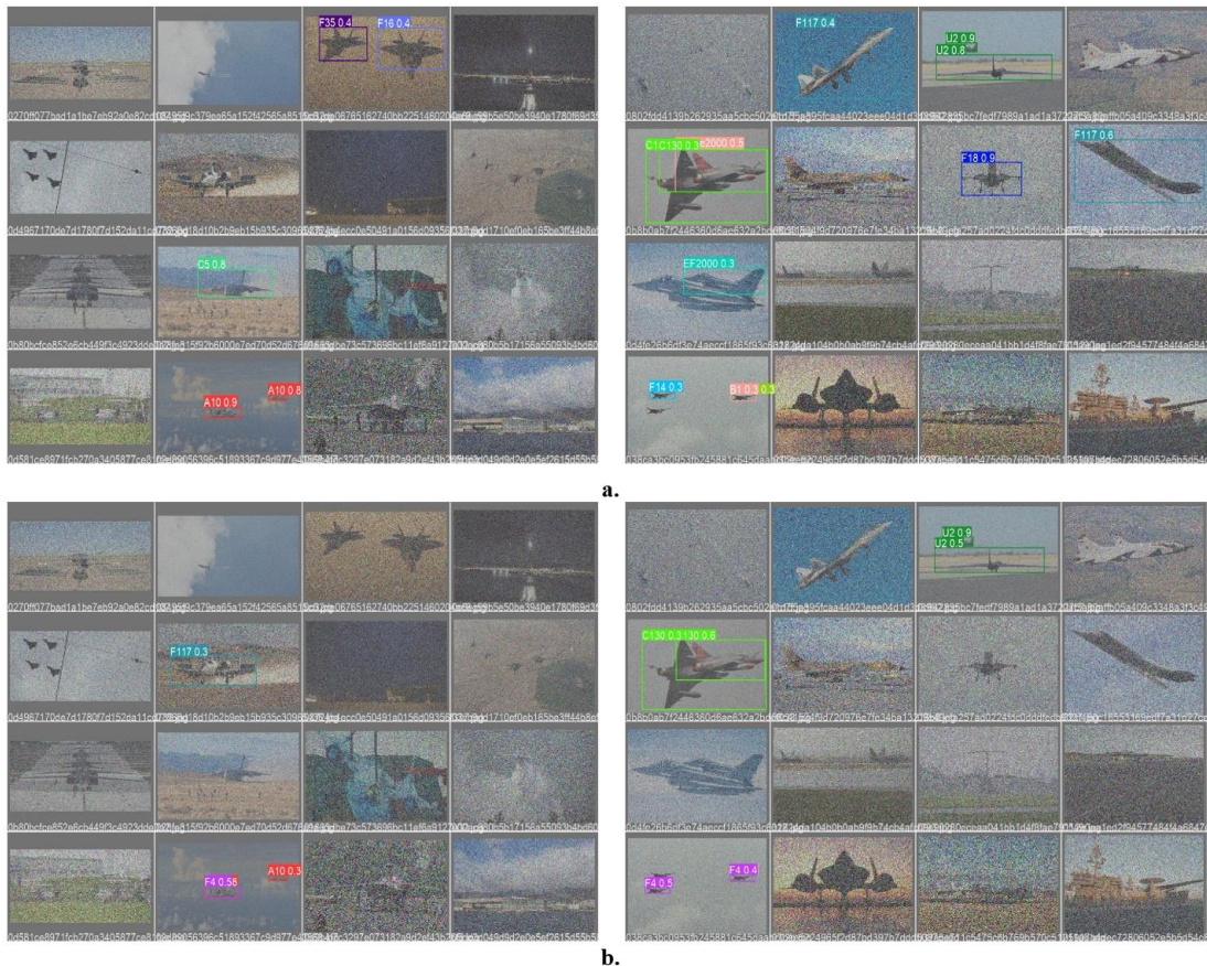
Figure 9. Examples of the YOLO detection on the 80% Gaussian-Dataset and 100% Gaussian-Dataset. a. 80% noise, b. 100% noise.
