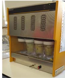
Figure 6. Soxhlet apparatus used for extracting oil.
