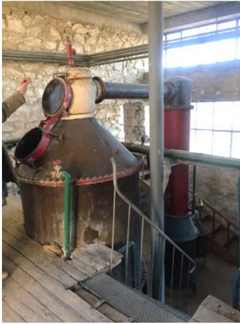
Figure 28: Gülbirlik Güneykent Rose Oil Factory Retorts in the interior.
