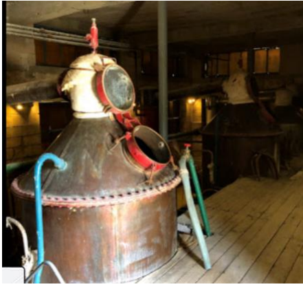
Figure 27: Gülbirlik Güneykent Rose Oil Factory Retorts in the interior.
