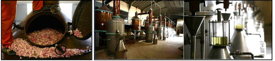
Figure 8: Loading Rose Flowers into Distillation Boilers, Steam Generator Powered Distillation Boilers.
