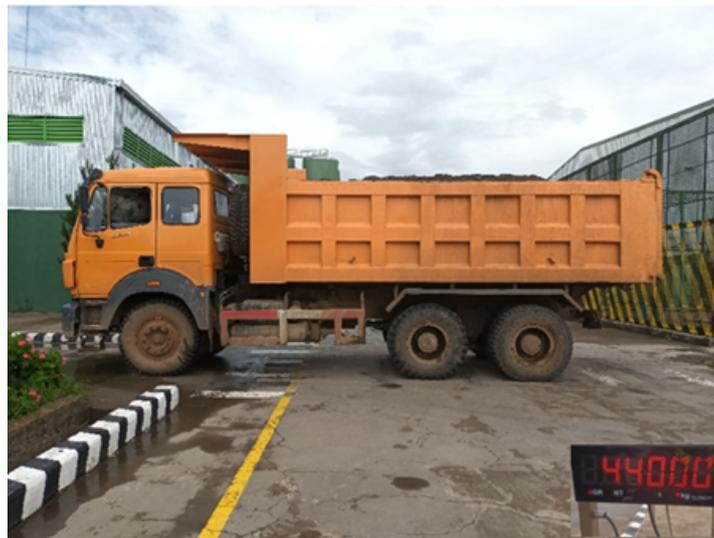
Fig. 5. Truck used for loading test - 44ton
