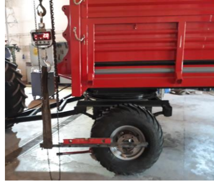
Figure 2. The test bench for measurement of the static brake torque
