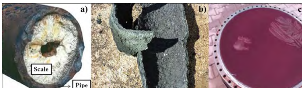
Figure 1-a) Scaling examples from some geothermal fields (Doğan et al., 2014), scale formation in b) Tuzla geothermal field and c) antimony sulfide (stibnite) scaling examples from geothermal fields obtained from Kübilay geothermal power plant.
