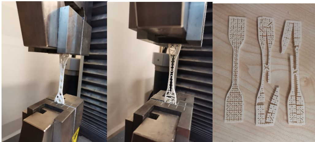
Figure 3. Application of the tensile test and the final state of the samples.
