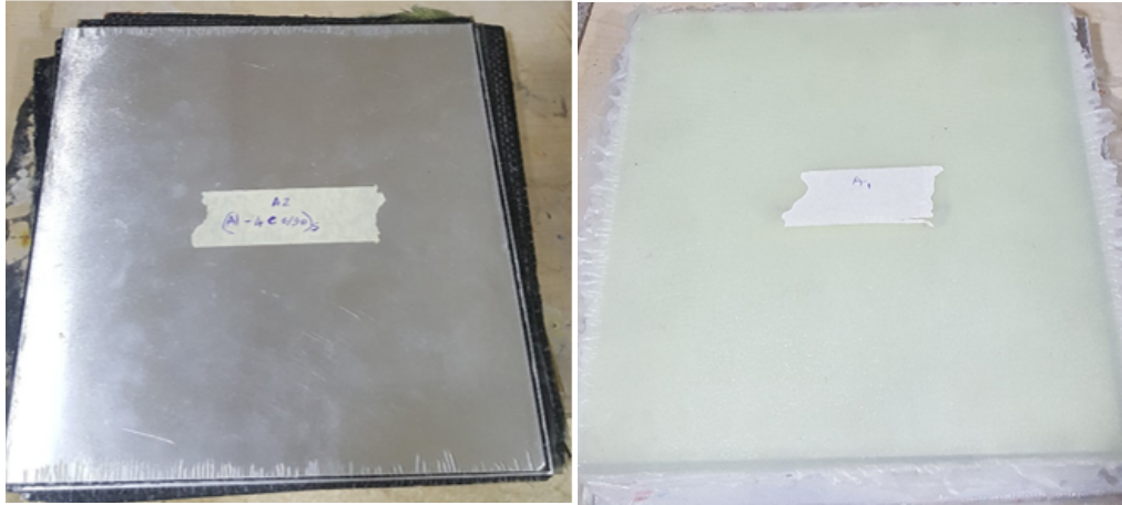
Fig. 1. FML composite plates manufactured: a) CARALL b) GLARE
