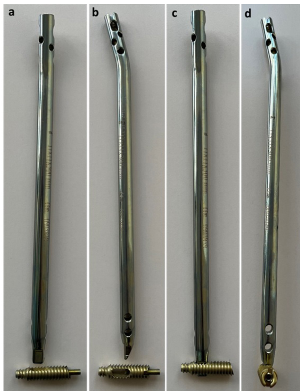
Figure 1. a: Coronal view of the DSBLS and the nail. b: The tibial nail in the sagittal plane and the entrance hole of the nail in the DSBLS. c: Locking of the tibial nail to the DSBLS in the coronal plane d: Locking of the tibial nail to the DSBLS in the sagittal plane
